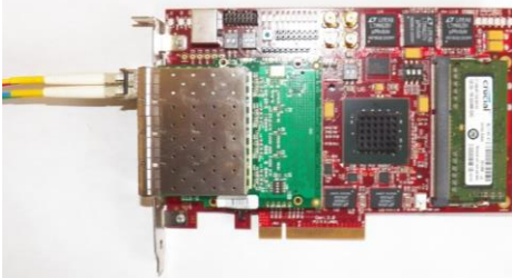
Data Transfer Controller (FPGA card with 8 SFP optical links)
