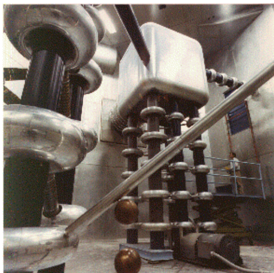
“Preac” - Static Cockcroft-Walton generator accelerates H - ions from 0 to 750 KeV.
